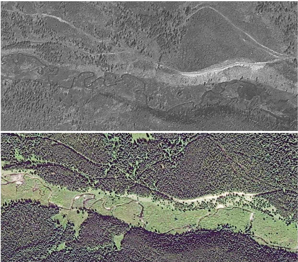
Photo 23. Comparison of historical (1949) and recent (2013) imagery of a section of Loomis Creek in the beaver meadows showing channel stability over 64 years.
